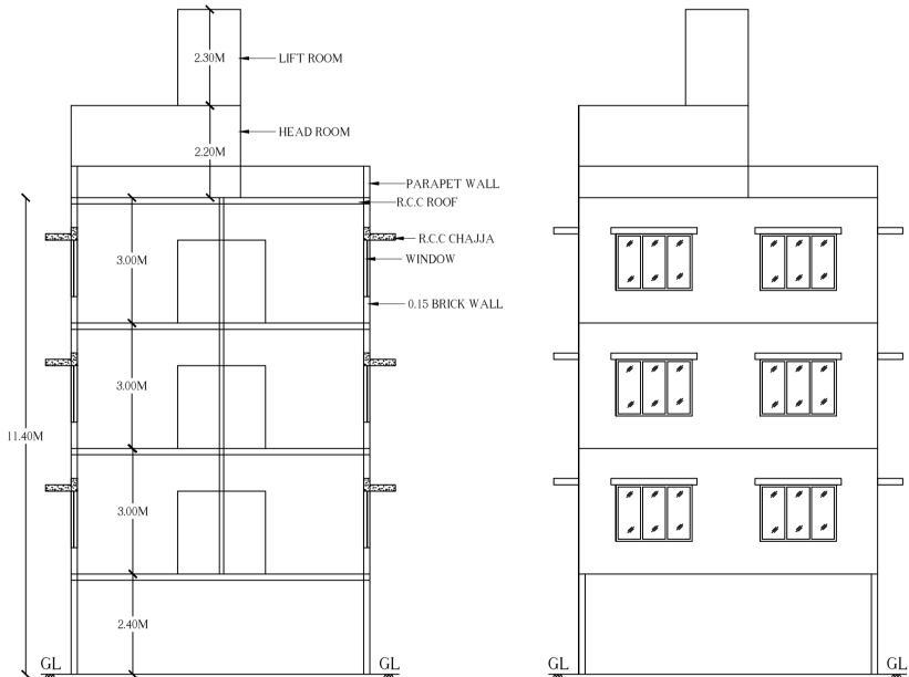
ELEVATION SECTION A-A
